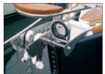
Bow fittings on some boats can be integrated with the bow anchor fitting.
