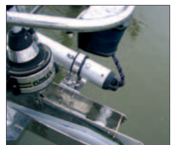
Side mounted installation on stem head anchor fitting
